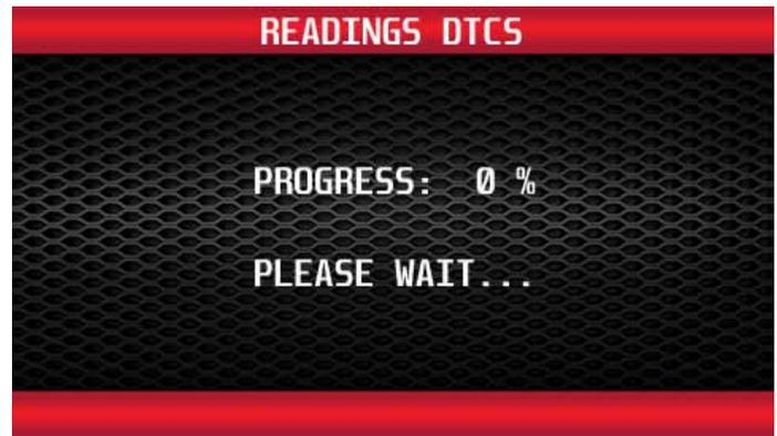
The programmer will immediately begin reading out the DTCs from the vehicle's computer. If no DTCs are present, the programmer will display the following message:
