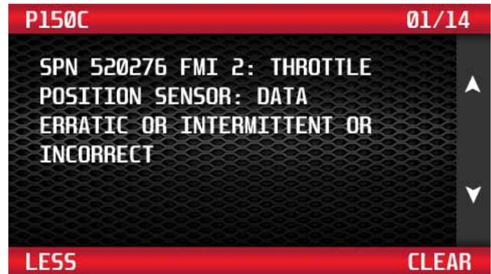
**NOTE:** Necessary repairs must be made to the corresponding DTC code(s) to properly clear the DTC(s). Make these repairs and clear all DTCs with the programmer **BEFORE** programming the vehicle.
