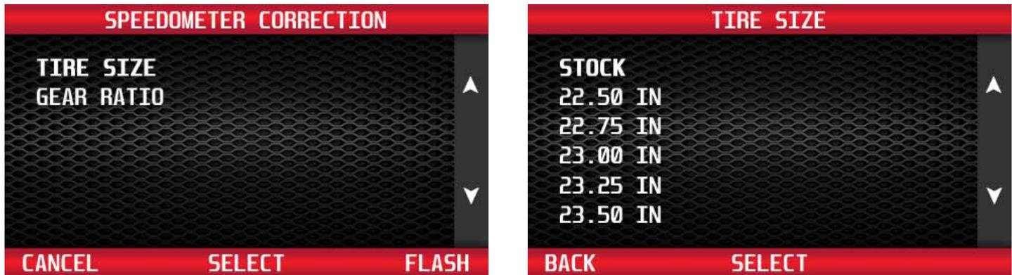
From the Speedometer Correction menu, use the buttons to the right of the screen to highlight Tire Size. Press the 'Select' button to recalibrate the speedometer reading for installed non-stock tire sizes. Use the buttons to the right of the screen to highlight the desired tire size. Press 'Select' to save the chosen value.
