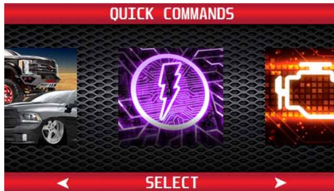
From the main menu, press the left or right arrow buttons and scroll to the Quick Commands icon. Press 'Select' to enter the Quick Commands menu.
