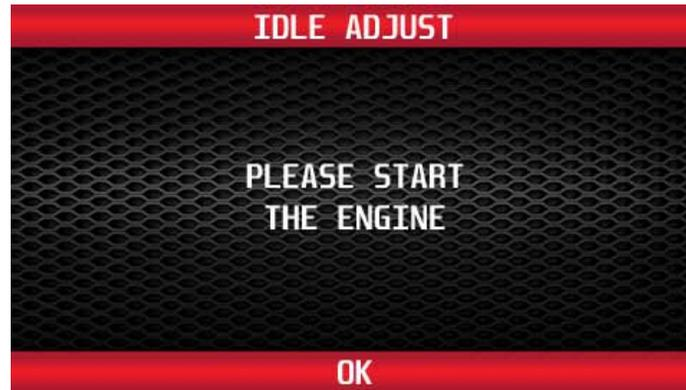
With the vehicle engine running, use the buttons to the right of the screen to highlight the desired idle RPM. Select the 'Back' button and the vehicle idle RPM will increase to the selected RPM.
