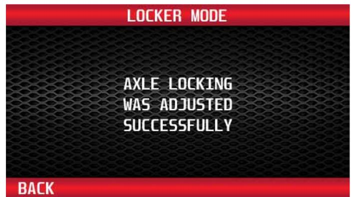
Select 'Adjust' to lock both the front and rear differentials. This will lock both front and rear below 20MPH. As you accelerate above 20MPH, the front disengages, above 30MPH, the rear disengages. When the vehicle speed drops below these thresholds, they automatically re-engage.
