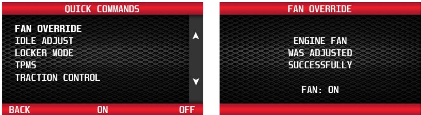
From the Quick Commands menu, use the buttons to the right of the screen to highlight Fan Override and press the 'On' button. This will manually override the engine fan cooling operation.
