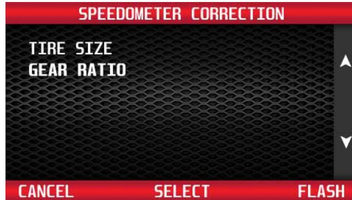
From the Speedometer Correction menu, use the buttons to the right of the screen to highlight Gear Ratio. Press the 'Select' button to recalibrate the speedometer reading for installed non-stock rear gear ratios. Use the buttons to the right of the screen to highlight the desired rear gear ratio. Press 'Select' to save the chosen value.
