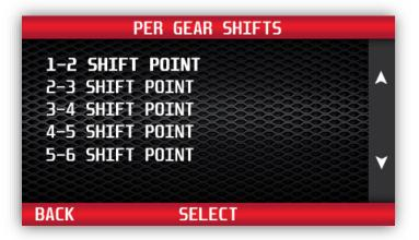
Press the 'Select' button, then use the buttons to the right of the screen to scroll up or down and highlight the value to increase or decrease the shift points. Press Select to save the chosen value.
