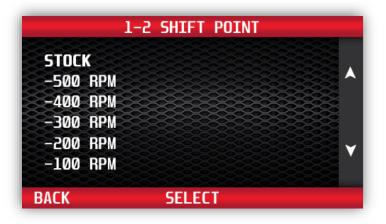
Press the 'Back' button to go back to the Gear Shift menu. Repeat the procedure above for each gear change. Once you have made the desired changes for each gear, press the 'Back' button to return to the Tuning Menu. For more information on Shift Points options, see Programming Features explanation in section 4.
