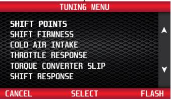
To adjust the shift points in all gears the same, select ALL from the Shift Points menu. To adjust the shift points for each gear change separately, select PER GEAR from the Shift Points menu.
