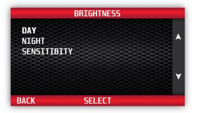
Use the buttons to the right of the screen to adjust the brightness of the display screen, from 1 to 10. Press the 'Back' button to return to the previous menu.
