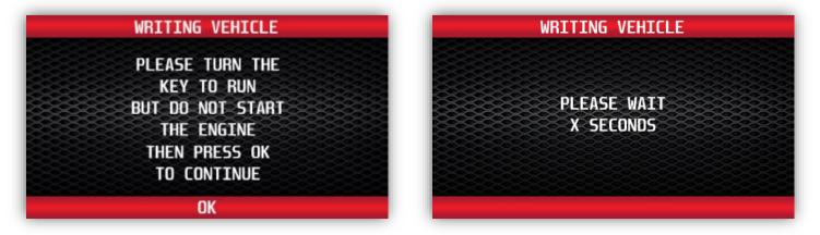
After the programmer has successfully programmed the vehicle, follow the instructions on the screen until you see the Successful screen.
