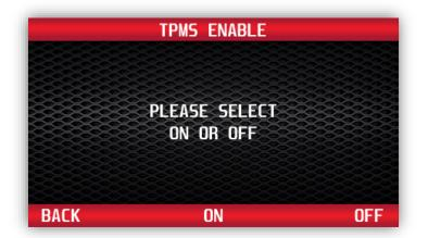
Press the button on the bottom to fully enable or disable the TPMS alarm.
