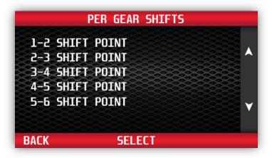
Press the 'Select' button, then use the buttons to the right of the screen to scroll up or down and highlight the mode to increase or decrease the shift firmness. Press 'Select' to save the chosen value.
