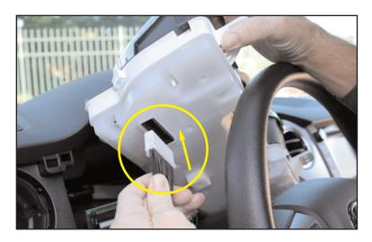
18. Reverse the process of these instructions to properly re-install the instrument panel components, as well as all other interior pieces removed for this installation.
