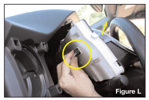
12. See Figure M. Remove the IPC by pulling it straight up behind the steering wheel.
