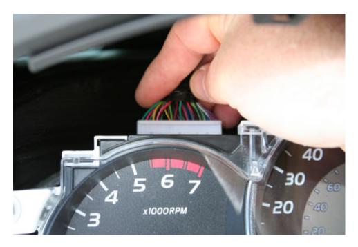
f. Using the supplied cable, connect the small black connector (C3) to the VSS inline module.
