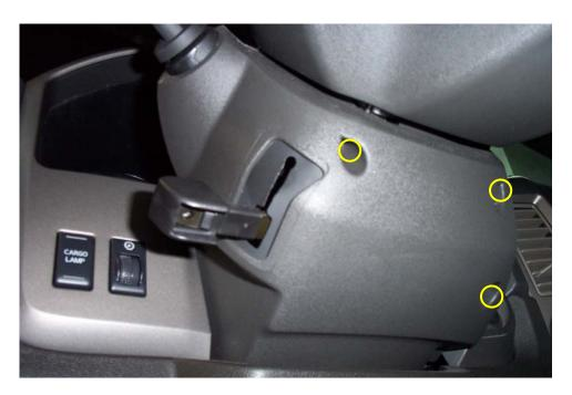
b. It will make it easier if you can remove the knob on the steering wheel angle adjustment lever. However, if it will not easily slide off, do not remove! The lower cover can be removed, but with the knob out of the way, the job is easier.
