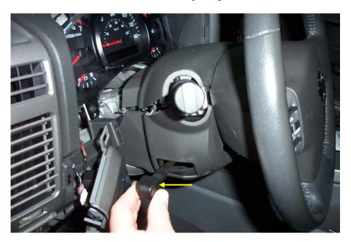
c. Remove the steering column covers. To keep from scratching the finish, you can wrap the end of the tool with painter's tape.
