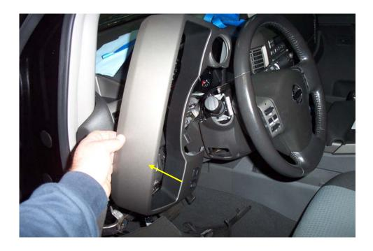
c. When it is fully separated, you can just rotate it around to the left hand side and lower it to rest on the floor board.
