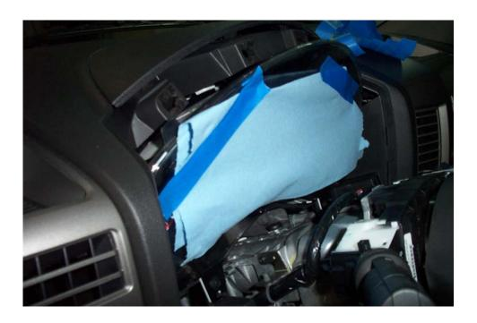
b. Use a 7mm socket to remove the 4 retaining screws which hold the Instrument Panel in place.
