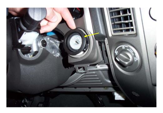
b. Starting on the driver's side, start separating the bezel from the dash.
