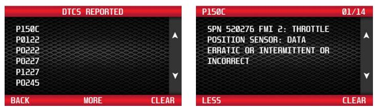
NOTE: Necessary repairs must be made to the corresponding DTC code(s) to properly clear the DTC(s). Make these repairs and clear all DTCs with the programmer BEFORE programming the vehicle.
