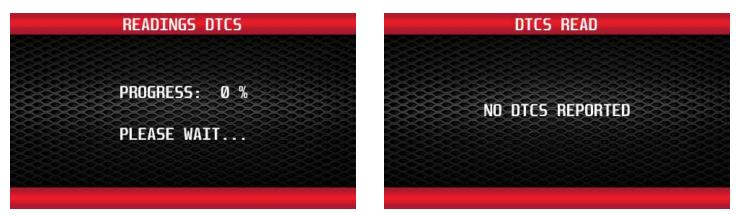
Prior to starting the programming process, the programmer will check for any Diagnostic Trouble Codes (DTCs). If any DTCs are present, the programmer will display them. You can review the DTCs before clearing.
