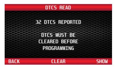
If the vehicle has no DTCs, the programmer will proceed immediately to Reading Vehicle mode.
