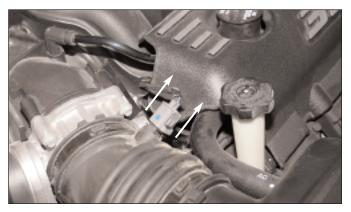
Disconnect the factory harness from the Intake air temp sensor.
