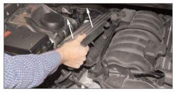
Lift off the engine cover (passenger side on SRT-8's). Ram Truck Specific: Disconnect the Intake Air Temp sensor. Then, using a flathead screwdriver or 8mm socket, loosen the clamp at the throttle body and lift the intake hose out of the way. Then remove the engine cover.
