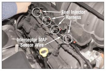
Route Interceptor MAP sensor harness under the fuel injector harness to the MAP sensor.
