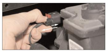
Disconnect the factory connector from the MAP sensor. This connector has a locking clip that must be slid back to unlock. Then, squeeze down the locking tab, and push the connector in slightly (toward sensor) and then remove.
