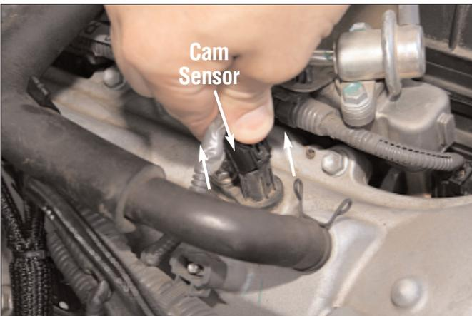
Disconnect the factory connector from the cam sensor. Push down on the connector, squeeze the release tab firmly, then pull up to remove the connector.
