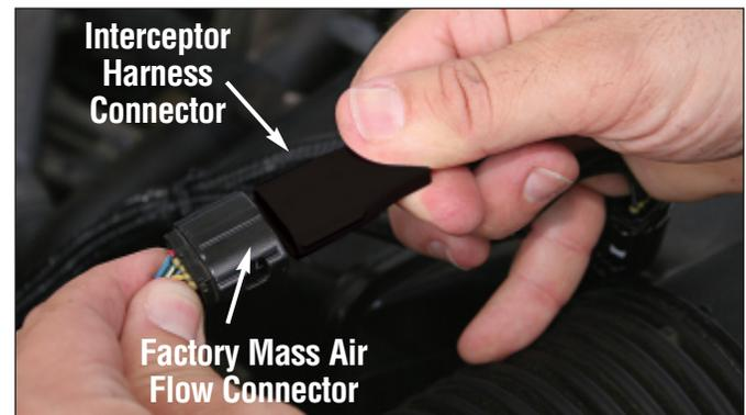
Plug the Interceptor harness connector into the factory Mass Air Flow connector.
