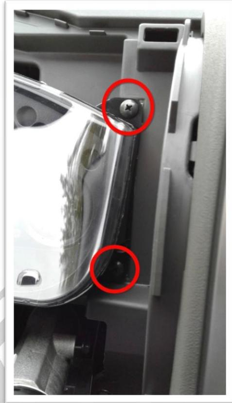
*Step 6b - Remove 2 Cluster screws on Right*
