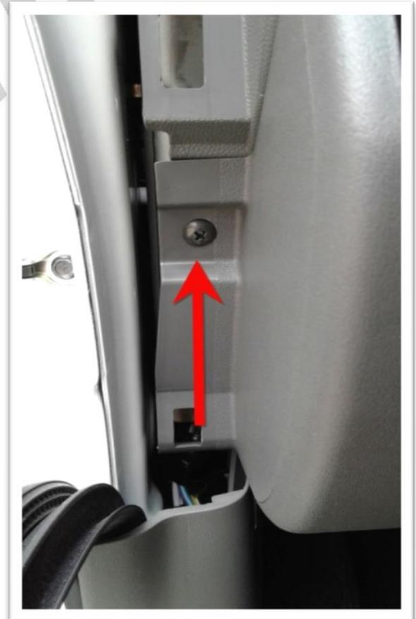
*Step 3 – Remove lower column shroud screw.*
