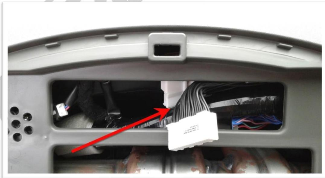
*Step 7a - Disconnect factory harness from Cluster. Connect this plug into Speedo Calibrator harness.*
