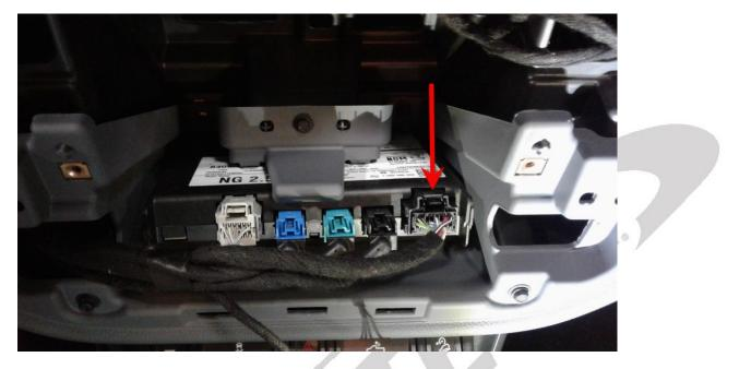
6. Plug the female end of the speedometer module harness in the vehicle's module.
