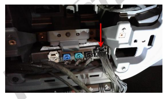
7. Insert the male connector of the speedometer harness into the factory vehicle harness, making sure to align the connectors so that both the retaining clips are facing up. Secure the 2 connectors with a zip-tie through the retaining clips. Be sure to not pull the zip-tie too tight to avoid damage to the clips.
