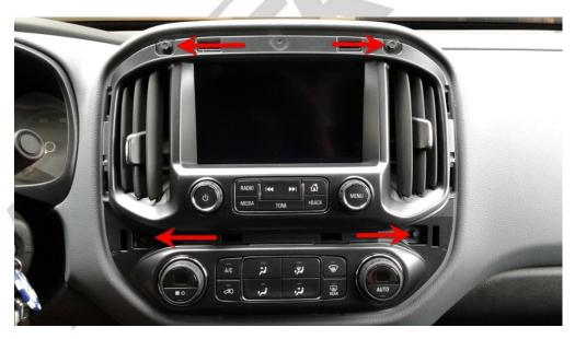
4. Sliding the center stack out, you will see (3) connectors on the back, disconnect #1 first. The tab for the #1 connector is very stiff, a small screwdriver or gloves might help.
