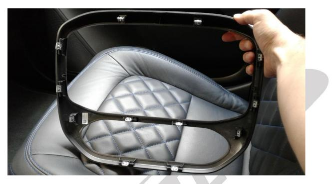
2b. Here is a visual of the location for the bezel's retaining clips.
