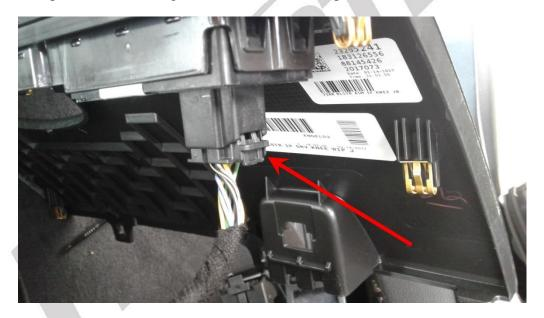
6. Look to the left of the steering column and you will see a module with 2 connectors. We will remove the black one by pulling the red locking tab back with a pick, small screwdriver or finger. Depress the tab in the middle and pull backwards to remove.
