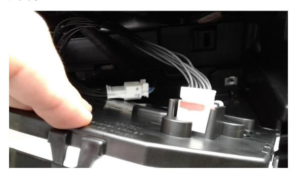
10c. Rest the module behind the main wiring harness for room and reinstall the I/C.
