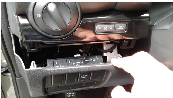
4. Insert the trim tool behind the bezel and push forward to release it. You do not have to disconnect the wiring harness.
