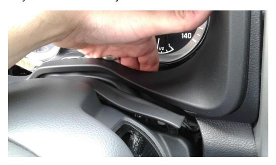
9. With access to the I/C achieved, remove the 3 phillips head screws. The cluster has small tabs that clip it in place, gently pull forward and it will come free.
