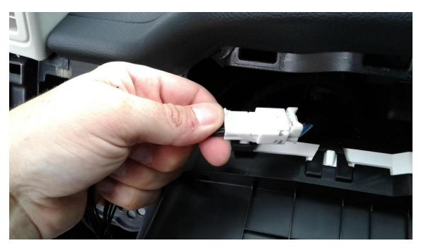
10b. Plug the male side of the Speedometer Module harness into the I/C.
