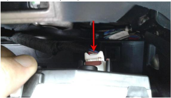
10a. Plug the factory I/C connector into the female side of the Inline Speedometer Module harness.
