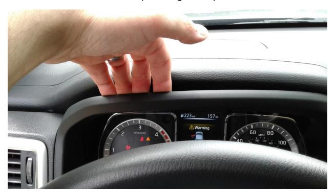
8. To remove the I/P shroud, you will need to disengage the vinyl steering column cover. Insert a small screwdriver on the left side and gently pry up to release the first clip.
