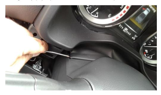
8a. Reach behind the shroud and with your fingers pull up on the steering column shroud until all of the clips are released. Once they are disconnected you can remove the I/P shroud.
