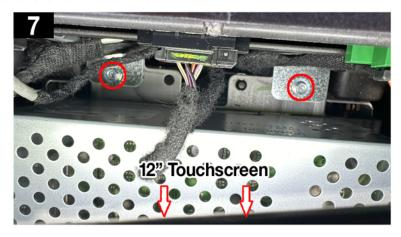
8. Remove the two (2) 7mm bolts on the upper area of the 12" touchscreen.
