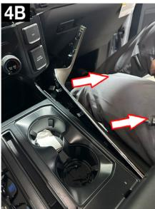
5. Remove the six (6) 7mm bolts holding the climate control panel in place. Gently pull the climate control panel away from the center console but DO NOT unplug any connectors.
