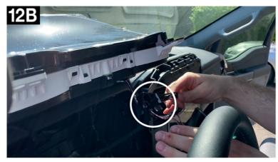
13. **Secure the In-Line Speedometer Calibrator Module.** Secure the In-Line Speedometer Calibrator Module and wires in place behind the instrument cluster using the provide zip ties.
