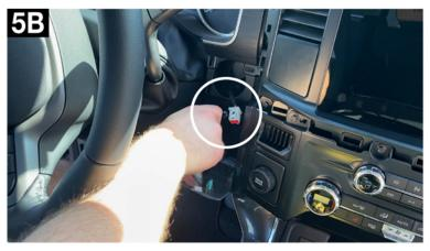
6. Remove the Steering Column Cover. Lower and extend the steering wheel position. Using the trim panel removal tool, pop loose the retaining clips on the steering column cover. This cover has six (6) snap-in retaining clips; four (4) on top and one (1) on each side near the bottom.
