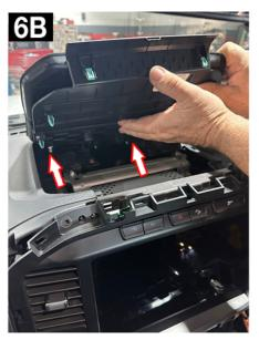
7. Remove the two (2) 7mm bolts located BEHIND the 12" touchscreen (center stack). **IMPORTANT NOTE: These bolts are hidden and will need to be removed in order to remove the 12" touchscreen.**
