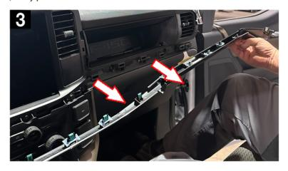
4. Using a trim removal tool or similar, firmly pull and remove the side console panels to access the climate control panel. Use caution to prevent breaking any clips.
