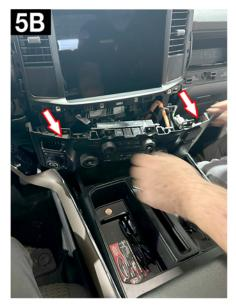
6. Remove the two (2) 7mm bolts holding dash tray in place. Then firmly pull up and remove the dash tray from the dashboard. Use caution to prevent breaking any clips.
