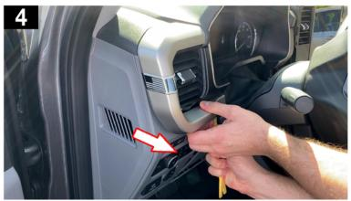
5. **Remove the Panel Screws.** Using a 7mm socket/nut driver, remove the cluster bezel screw to the left of the steering wheel. Once complete, remove the two (2) screws to the right of the steering wheel which are side-by-side just below the ignition switch location. These screws are tightened to 22 Lb.In (22.5Nm) when re-installed.
