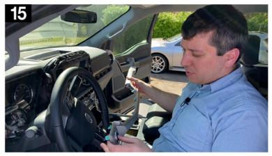
16. **Drive the Vehicle and Verify the Speed.** Prior to fully reinstalling the rest of the interior panels it is advised to drive the vehicle to verify that the speed readings are correct. You can use a GPS reading from your cell phone to compare the dash speed reading. Do this test in a safe environment with little traffic to ensure your safety and those around you.
