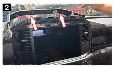
3. Using a trim removal tool or similar, firmly pull out and remove the lower bezel below the touchscreen. Use caution to prevent breaking any clips.
