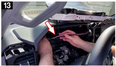
14. **Install the Instrument Panel Cluster.** Carefully lower the instrument panel cluster back down into place with the screws you removed in Step 8. We recommend getting all four (4) of the screws installed, but not fully tightened. Before tightening completely, push the cluster in all the way and then tighten the screws down to 22 lb.in (22Nm).
