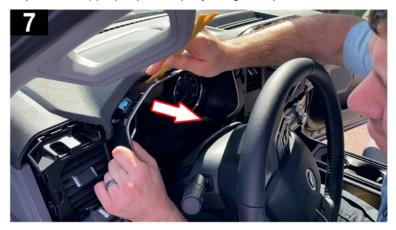
8. Remove the Instrument Panel Cluster. Using a 7mm socket/nut driver, remove the instrument panel cluster screws at each corner of the cluster. These screws are tightened to 22 Lb.In (22.5Nm) when re-installed. Once removed, gently lift the cluster out and set it lightly on the dash with the dials facing up.
