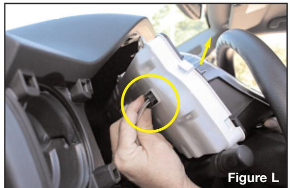
12. See Figure M. Remove the IPC by pulling it straight up behind the steering wheel.
