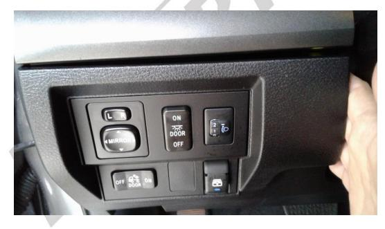
5. Reach under the grey trim panel and pull backwards to release it. Doing this should release the A/C Vent Register, if it does not gently pry underneath to release it.
