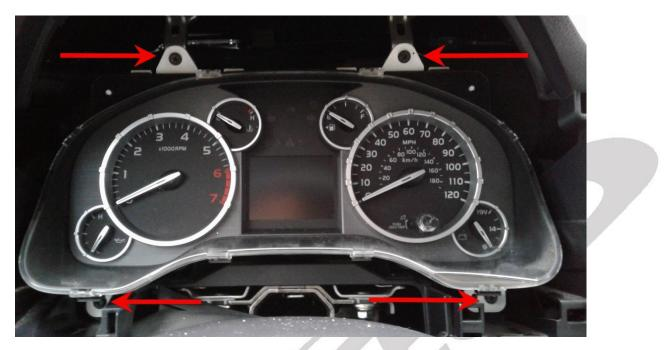
8. Remove the (4) 10mm/Phillips Head Screws that retain the I/C.
