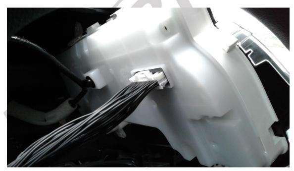
12. Tuck the Speedometer Calibrator module and harness back behind and to the left of the I/C. Clearance is limited but adequate.
