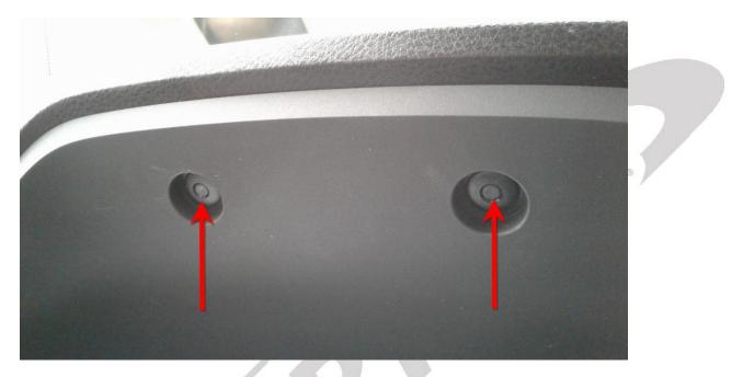
7. Once the shroud is unclipped, gently lay it down to gain access to the vinyl column cover. There are small clips that can be pressed with your fingers that will release the cover. Work each one out by pressing one side then the other.
