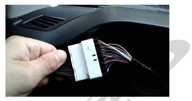
10. Take the Speedometer Calibrator harness and insert the factory I/C harness into the male end.
