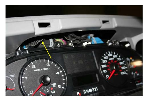
7. Re-install the Instrument Cluster and reverse the process of the procedures to re-install the Instrument panel.
