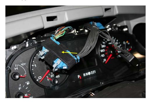
d. Connect C1, of the supplied harness, to the instrument panel cluster. Then tuck the harness and module above, and behind the instrument cluster.
