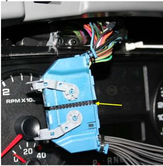
c. Using the supplied Velcro, or hook-and-latch, bind the connectors as illustrated in the following photo.
