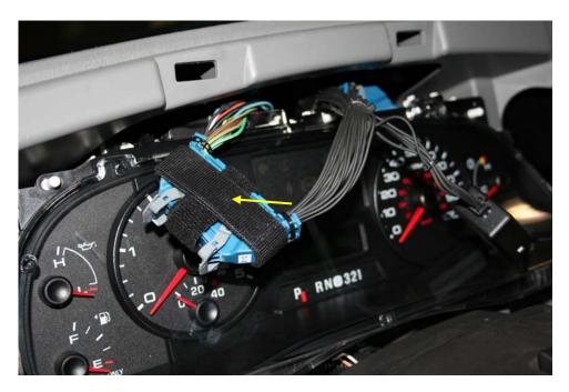
iv. Connect C1, of the supplied harness, to the instrument panel cluster. Then tuck the harness and module above, and behind the instrument cluster.
