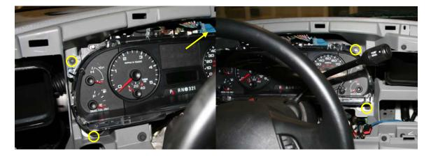
1. Look to the top of the connector, you will see a Grey lever. Press the button, and pull the lever up and back at the same time. After the lever is pulled back, the connector should easily release from the Instrument Panel.
