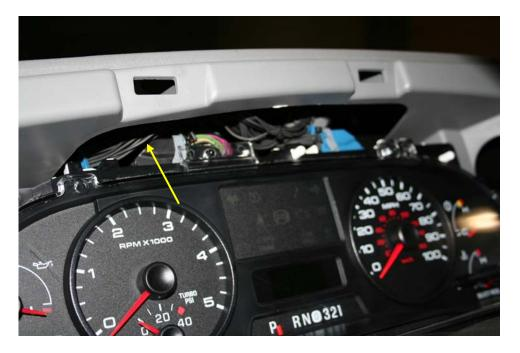
f. Re-install the Instrument Cluster and reverse the process of the procedures to re-install the Instrument panel.
