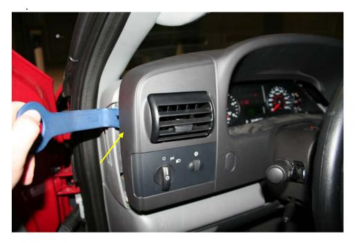
b. Disconnect the head light switch, dimmer switch, and 2WD/4WD switch connectors from the back of the panel
