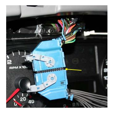
iii. Using the supplied Velcro, or hook-and-latch, bind the connectors as illustrated in the following photo.
