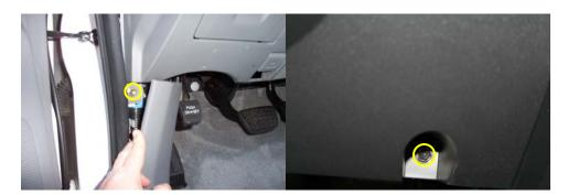
c. Separate the lower instrument panel cover and lower it to the floor. As you pull the panel out on the right hand side, the ignition key bezel will pop out. Later, when you re-install the panel, you simply press the ignition key bezel back into place.
