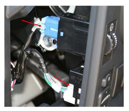
b. Using your fingers or trim tool, gently pull out on the finish panel, then rotate it upward and to the left, then lay it towards the floor, or if you removed the connectors, just remove the panel.
