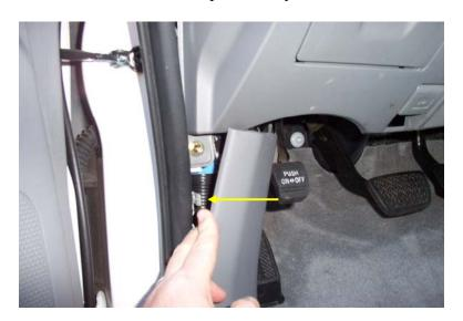
b. It's not necessary, but it makes room, while removing the lower instrument panel to pull the door seal out and away from the instrument panel. This allows room to get your fingers or trim removal tool behind the panels.
