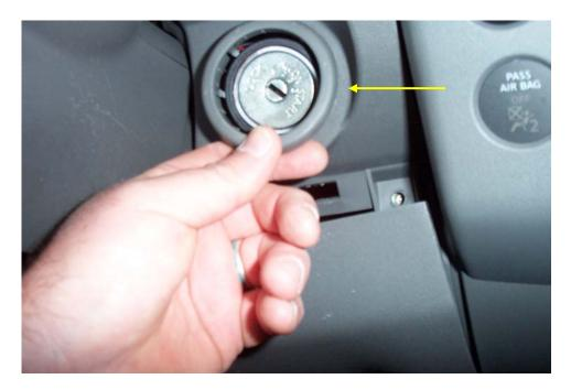
8. Remove the upper steering column cover. There are 2 Phillips head screws; remove them and use a tool like the one below to separate the column covers. To keep from scratching the finish, you can wrap the end of the tool with painter's tape.
