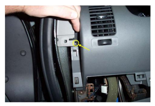
7. Remove the Ignition switch bezel.
