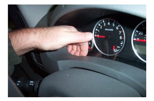
b. Gently twist the upper portion of the side trim to expose the outer tabs of the upper instrument panel bezel. This will assist you in removing the bezel.
