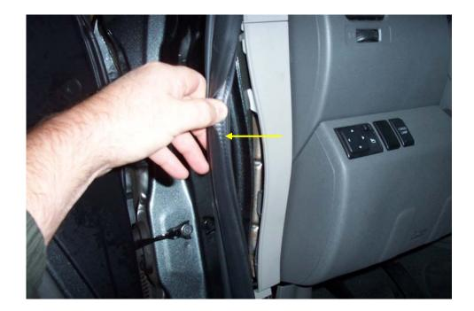
4. With the rubber trim pulled away, use a trim tool to help get behind the side trim piece, shown in the photo, then remove the piece by evenly exerting outward pressure. Only remove the lower piece.
