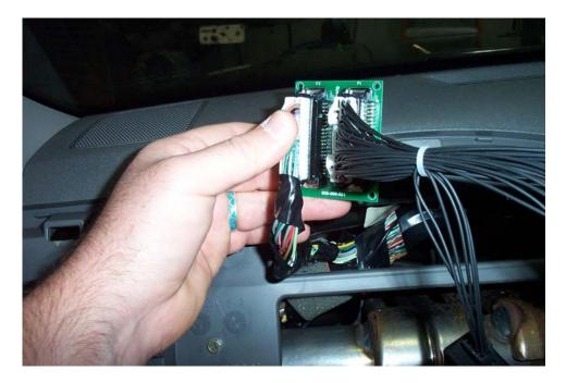
14. Carefully stow away the inline module and the green interface board.
