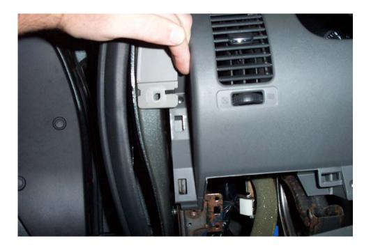
10. Using a Phillips screwdriver, take out the 4 retaining screws to remove the Instrument Panel. After the screws are removed, press the release tab on the electrical connector and gently pull it from the instrument panel.
