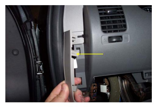
5. Using your fingers, carefully separate the lower Instrument Panel trim bezel. There are electrical cables connected on the left hand side, when removed, lower it to the floorboard. (To lower the right hand side, it helps to tilt the steering wheel up and separate the panel from below the steering wheel.)
