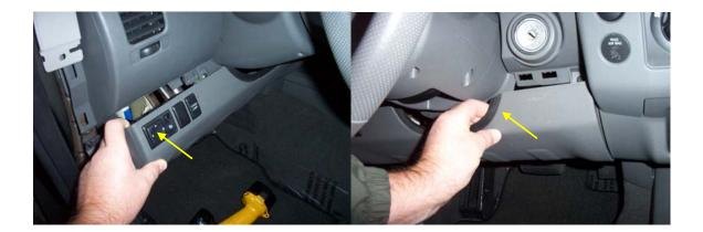
6. With the Phillips screwdriver, remove the retaining screw on the left-hand side of Instrument panel upper bezel
