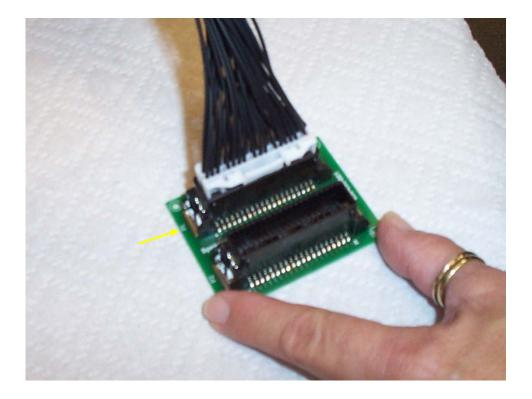
13. Connect the vehicle's Instrument Panel connector to P2 of the green interface circuit board.
