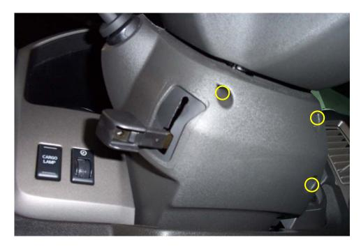
b. It will make it easier if you can remove the knob on the steering wheel angle adjustment lever. <u>However, if it will not easily slide off, do not remove!</u> The lower cover can be removed, but with the knob out of the way, the job is easier.
