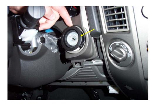
b. Starting on the lower left hand side, separate the bezel from the dash.
