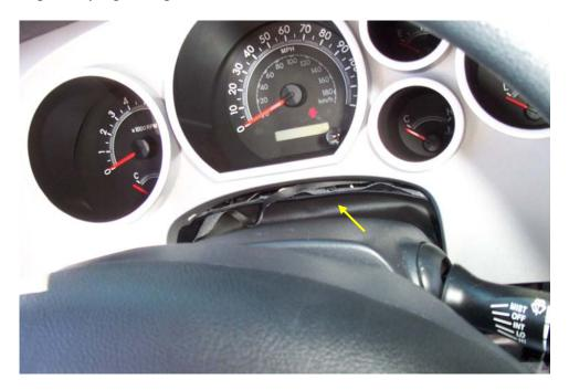
d. Utilizing the openings in the bezel, use your fingers to press the locking mechanisms to release the curtain from the bezel.
