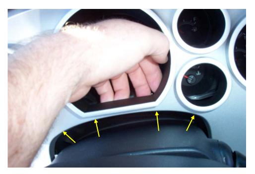
6. Utilizing a 10mm tool, remove the retaining bolts from the IPC. Pull the unit forward and disconnect it from the harness. Note: To prevent breaking the connectors, DO NOT rock the connector back and forth. Squeeze the release and pull straight out.
