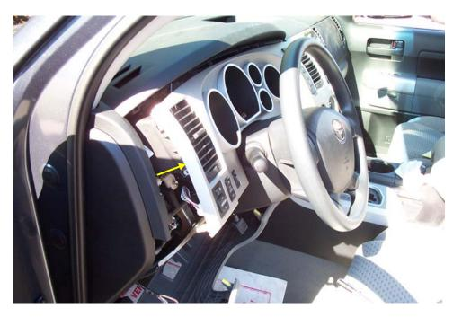
b. While peering behind the upper IPC panel bezel, you will need to disconnect two connectors. Note: To prevent breaking the connectors, DO NOT rock the connector back and forth. Squeeze the release and pull straight out.
