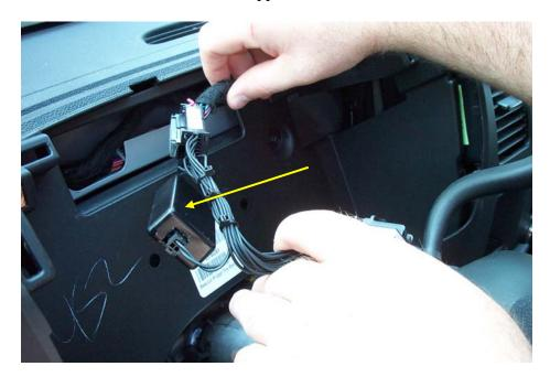
d. Stow the harness assembly, except for C1, into the back area as shown below.
