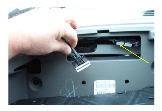
e. Connect C1 of the supplied harness to the Instrument Panel Cluster.
