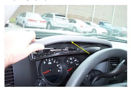
c. Using the 7mm socket, remove the two retaining screws, then separate the bezel and remove it from the dash.
